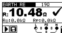
Figure 5.35: Example of earth resistance measurement result
